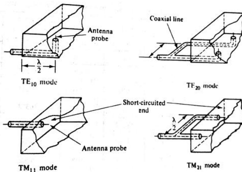
The methods of excitation for various modes in rectangular waveguides are shown in Figure.
