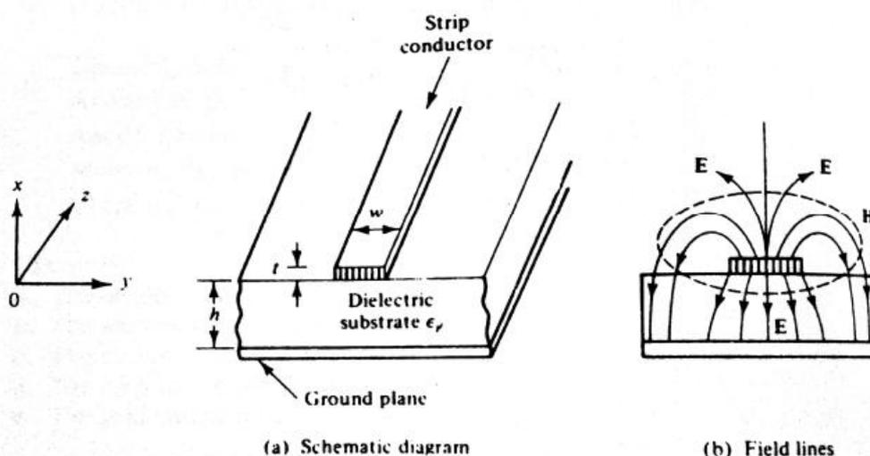
The theory of TE or TM coupled lines applies as an approximation only. The approximate field distribution is shown in the above Fig in b, where as a is the schematic diagram of the microstrip line.
