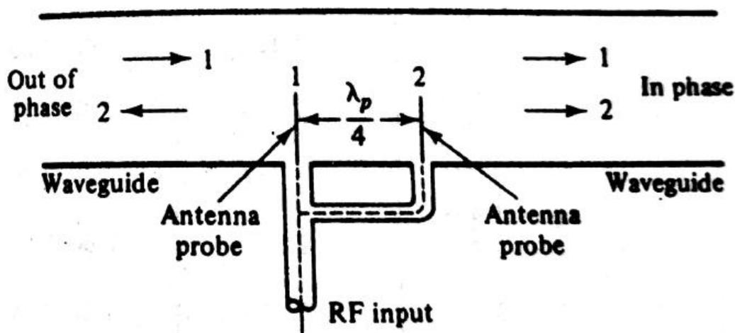
The field intensities radiated by the two antennas are in phase opposition to the left of the antenna and cancel each other, whereas in the region to the right of the antenna, the field intensities are in time phase and reinforce each other. The resulting wave thus propagates to the right in the guide.
