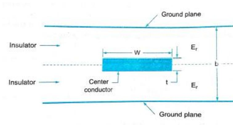
loss dielectric substrate ( $E_r$ ). The substrate is between two metallic ground plates, the width of the ground plates being five times the spacing 'b' between
