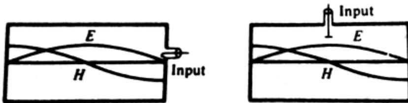
The figure shows the method of excitation for the rectangular resonator. The maximum amplitude of standing wave results when the frequency of the impressed signal is equal to the resonant frequency.
