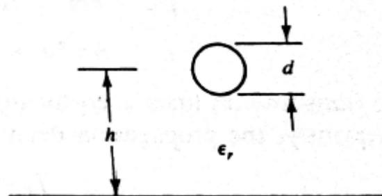
The characteristic impedance of a wire –over-ground line is given by
