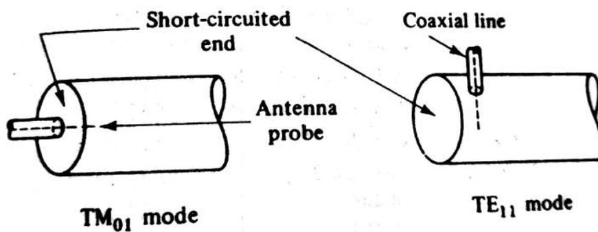
A common way to excite TM modes in circular waveguide is by a coaxial line. At the end of the coaxial wire a large magnetic intensity exists in  $\varphi$  direction of wave propagation. The magnetic field from coaxial line will excite the TM modes in the guide.
