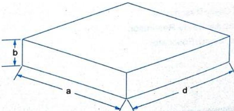
In general, a cavity resonator is a metallic enclosure that confines the electromagnetic energy. The stored electric and magnetic energies inside the cavity determine its equivalent inductance and capacitance. The energy dissipated due to the finite conductivity of the cavity walls determines the
