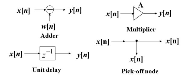
A realization is **canonic** if the realization uses minimum number of delay units. Two realizations are equivalent if they have the same transfer function.
