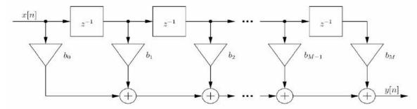
Here, the filter has an order of M, it requires M delays/memory locations, M+1 Multipliers, and M adders.
