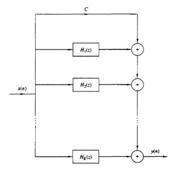
Each of the subsystems can be realized either in  $Direct\ Form\ II$ , or  $Direct\ Form\ II$  or transposed form.
