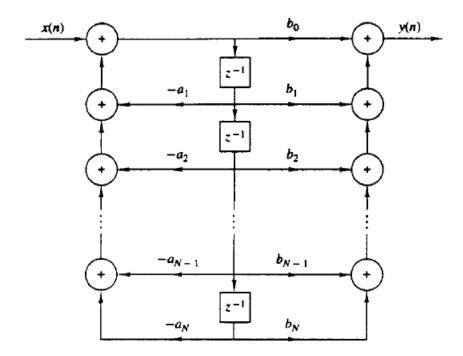
This structure requires M+N+1 multipliers, M+N additions and maximum  $\{M, N\}$  delays. Since this structure minimizes the number of delays, it is called **canonic.**
